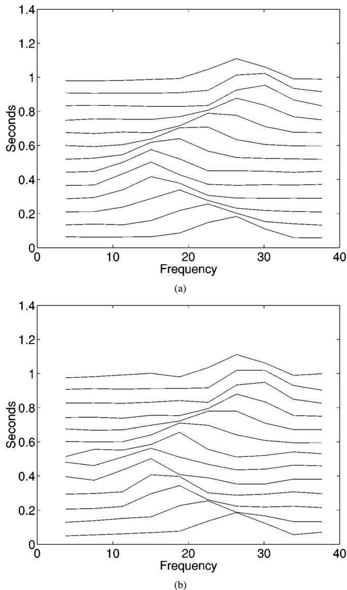
Fig. 4. Short-time fourier transform estimates of the spectrogram for (a) the low noise variance data in Fig. 2 and (b) the high noise variance data in Fig. 3. To achieve a reasonable temporal resolution the STFT trades off spectral resolution.
