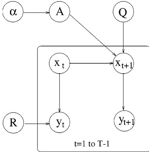
Fig. 1. Nonstationary autoregressive model. The autoregressive coefficients  $x_t$  are modeled as a linear dynamical system. The precision of the observations is given by  $R$  and the coefficients evolve deterministically via the transform  $A$  and stochastically via additive noise with precision  $Q$ . Each element of  $A$  has prior precision  $\alpha$ .
