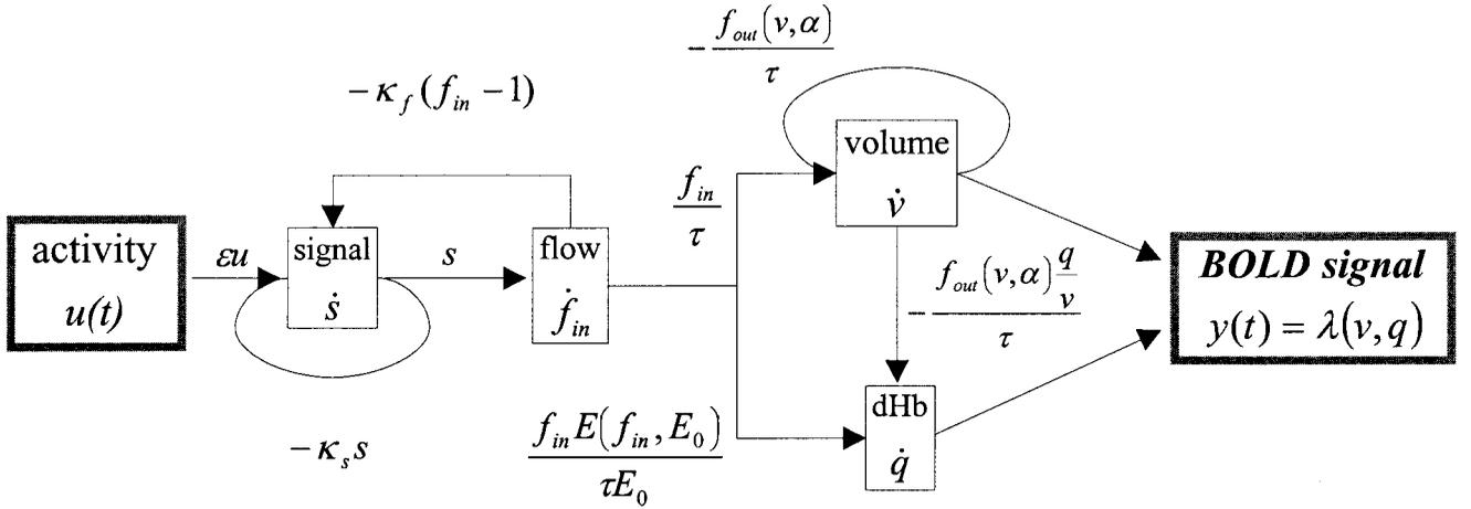
**FIG. 1.** Schematic illustrating the architecture of the hemodynamic model. This is a fully nonlinear single-input  $u(t)$ , single-output  $y(t)$  state model with four state variables  $s$ ,  $f_{in}$ ,  $v$ , and  $q$ . The form and motivation for the changes in each state variable, as functions of the others, is described in the main text.
