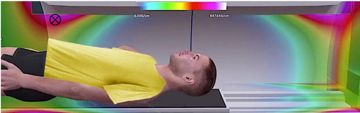
Derivative of the main magnetic field: \partial B_0 / \partial z
