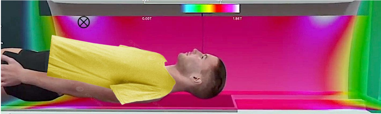
Derivative of the main magnetic field: \partial B_0 / \partial z
