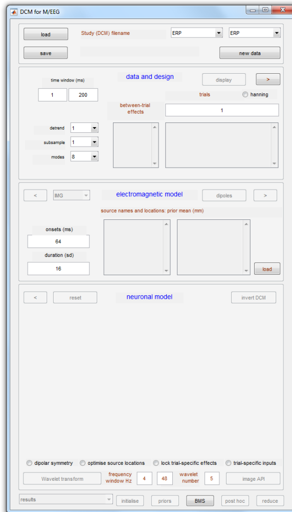
Figure 39.9: The Dynamic Causal Modeling GUI splits model specification into three reversible phases (i) data and design, (ii) electromagnetic model and (iii) neuronal model. One can move forwards and backwards in the model specification using the left and right arrow buttons (these become highlighted when sufficient information has been entered to proceed to the next step).
