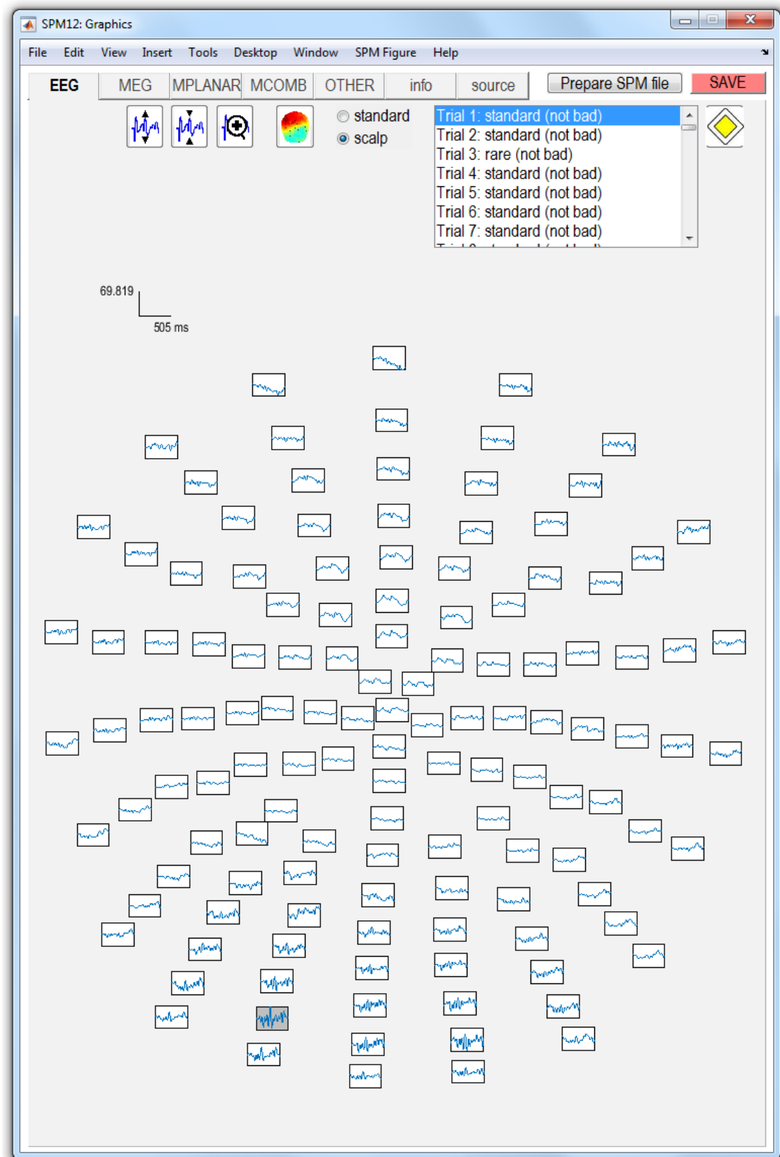
Figure 40.1: Scalp topography of single trial MMN EEG data. Channel 14, second-row from bottom, left hemisphere contains (slightly) higher variability data than the others. This channel is to be marked as artefactual (ie. 'bad').
