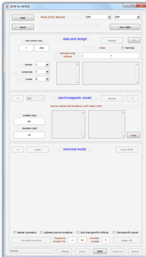
Figure 40.9: The Dynamic Causal Modeling GUI splits model specification into three reversible phases (i) data and design, (ii) electromagnetic model and (iii) neuronal model. One can move forwards and backwards in the model specification using the left and right arrow buttons (these become highlighted when sufficient information has been entered to proceed to the next step).
