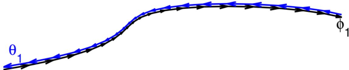
Decompose a curved path into a series of short line segments, and add the lengths of the segments together.
